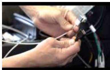
23. Plug the OEM charging/data cable of the smartphone to the USB extension cable.
