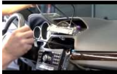
14. Run the LVDS cable into the radio cavity.
