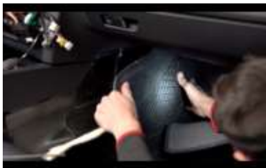
16. Fold back the carpet on the left side passenger footwell.
