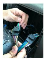
3. Plug the male connectors of the BTGM-33 T-harness to the radio.
