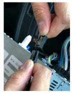
5. Run the microphone wire along the front headliner, down the A pillar and towards the radio. Plug the 3-pin plug of the microphone cable to the mating connector on the BTGM-33 T-harness.
