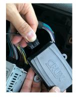
6. Plug the 12-pin Molex connector to the BTGM-33 module.
