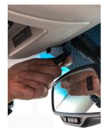
4. Mount the microphone to a desired location. We recommend mounting it by the rearview mirror or the A pillar. Point the microphone towards the driver.
