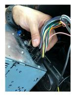
2. Unplug the factory radio connectors and plug them into the BTGM-33 T-harness.
