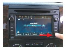
9. Press the SEEK DOWN button until you hear a beep to toggle between XM and Bluetooth mode. When a phone call is received, the BTGM-33 will automatically change to BT mode even if the radio is in any other source.
