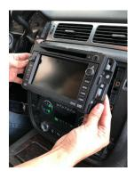
1. Remove the radio to gain access to the connectors.
