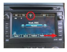
8. Go to XM mode on the radio and press SEEK DOWN ⋈ until you hear a beep. Confirm that blueLOGIC is shown on the screen. Play music from your phone and the audio will be heard from the factory speakers. Make a phone call to confirm that the handsfree mode is functioning.
