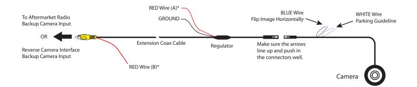
\*NOTE: To power the camera, use RED Wire A or B. If tapping power from the radio or RVC Interface, make sure to insulate RED Wire A to avoid it from shorting. If you will be tapping power from the reverse light +12V, insulate RED Wire B to avoid it from shorting. With either connection the Black GROUND wire needs to be connected to a solid chassis ground. For vehicles with manual transmission, we recommend tapping +12V power from the reverse light.
