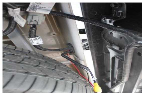
8. Run the cables through the hole on the bed and under the bed of the truck. We recommend running the cable under the passenger side of the truck bed.
