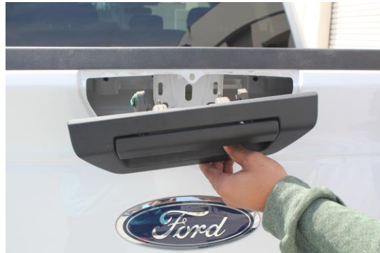
6. Carefully remove the tailgate handle assembly by lifting the handle and pulling slightly upward. Remove the OE lock and install it on the CFD-15KM.
