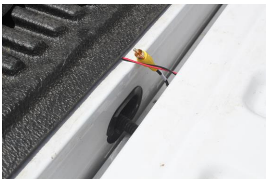
7. Fish the video and power cables inside the tailgate towards the bed of the truck.
