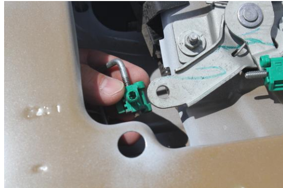
4. Remove the latch rod by pressing in the locks on the sides then pull back.
