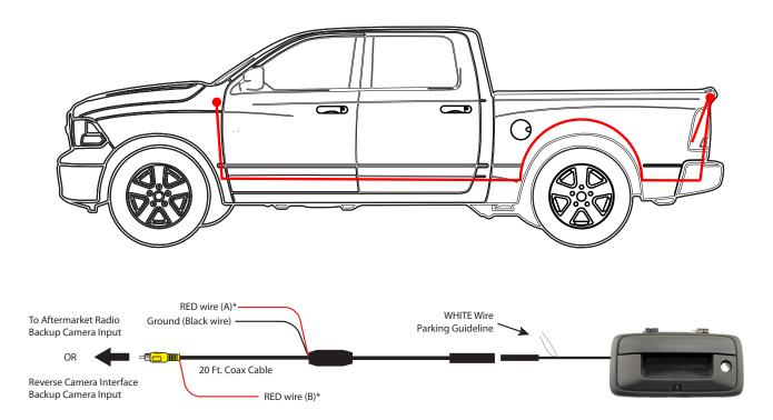
**\*NOTE:** To power the camera, use RED Wire A or B. If tapping power from the radio or RVC Interface, make sure to insulate RED Wire A to avoid it from shorting. If you will be tapping power from the reverse light +12V, insulate RED Wire B to avoid it from shorting. With either connection the Black GROUND wire needs to be connected to a solid chassis ground. For vehicles with manual transmission, we recommend tapping +12V power from the reverse light.
