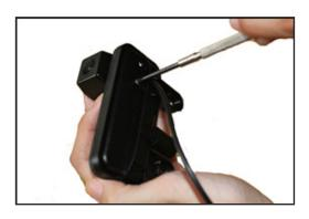
2. Remove the 4 screws holding the CMB-15T camera.
