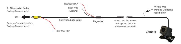
\*NOTE: The camera needs a +12V trigger. Power the camera at the headunit using RED Wire B or from the reverse light wire using RED Wire A. <u>DO NOT</u> connect both wires to +12V at the same time. Insulate the red wire that is not being used. Tap the Black wire to an existing ground lead, or ground Black wire securely to vehicle body metal.
