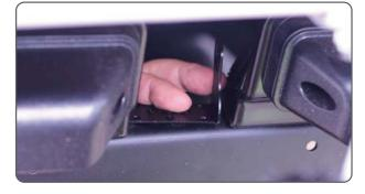
4. Install the camera to the bracket. Do not completely tighten the screws yet.
