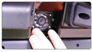
6. Mount the transmitter no more than 3 feet from the camera.
