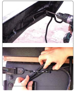
18. Connect receiver's red wire to ACC and black wire to ground. Plug the Yellow video RCA to the monitor (not included).
