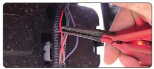
15. Tap the red and black wires of the CTR-01Q camera cable to the positive and negative wires.
