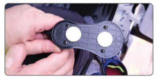
20. With the ignition turned to ACC, put the vehicle in reverse. Turn on the monitor and find the best direction for the receiver turning it until you see atleast 3 bars on the monitor.
