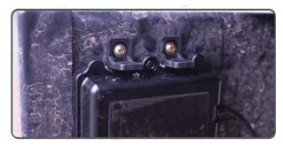
12. We recommend putting silicone sealant around the base of the transmitter to prevent dirt from going behind the transmitter.
