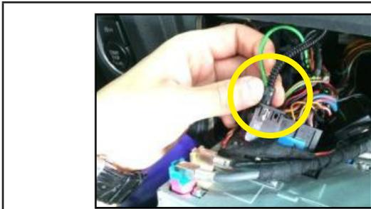
1. Remove the headunit and unplug the Quadlock connector. Unplug the Fiber Optic cable connector from the main connector housing.
