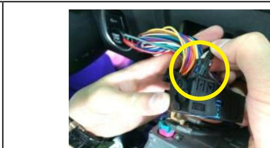
2. Plug in the fiber optic cable connector to the female Quadlock connector supplied on the MRVBM-77Q power harness.
