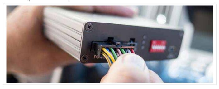
Step 4 - After connecting the module, set the proper dip switches to the "ON" position. Make sure to set the AV sources being used to the "ON" position. NOTE: The Video In-Motion feature does not require activation. This feature is permanently ON and will not disturb the navigation GPS performance.
