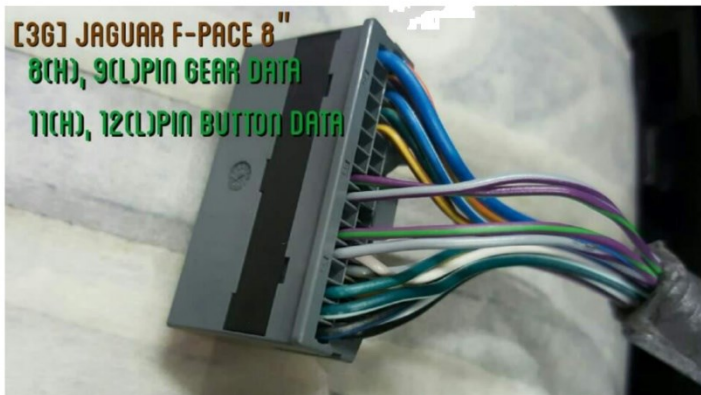
The CAN wires on a Jaguar F-Pace can be found at the 32-pin connector located behind the air conditioning unit.
