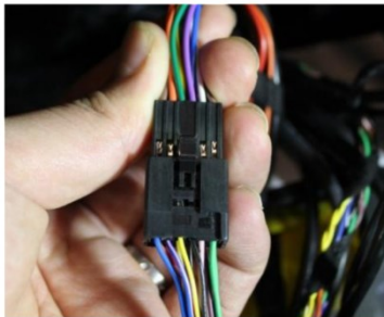
Plug the inner female 12-pin connector to the mating end of the CAN IN/OUT cable provided
