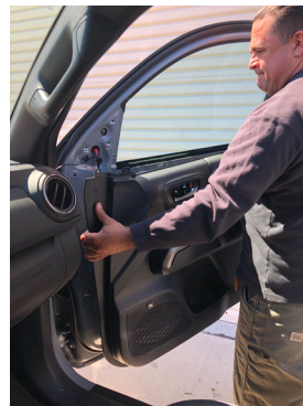
4. Unhook the door panel by pulling it upward. Unplug the speaker and doorlock harness.
