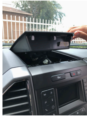
2. Remove the tray and remove the 2 screws holding the radio bezel.
