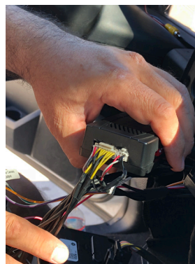
6. Plug the white, 18-pin connector of the T-harness to the RFM-FD4 module.
