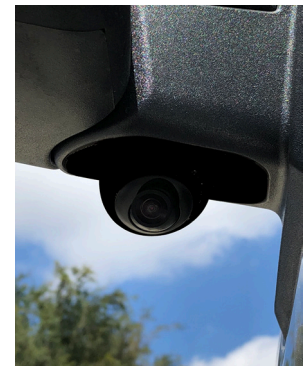
6. Tuck in the camera cable inside the cavity and snap in the CSV-FD15 side mirror cover with camera.
