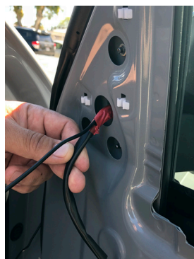
5. Use a fine hooked pick tool to remove the OEM side mirror cover. Fish the camera cable through the hole.
