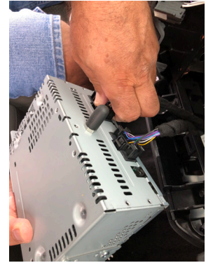
4. Remove the radio, unplug the 12-pin connector and plug it into the RFM-FD4 T-harness. Plug the other end of the T-harness to the radio.
