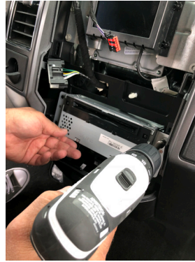
4. Remove the radio, unplug the 12-pin connector and plug it into the RFM-FD4 T-harness. Plug the other end of the T-harness to the radio.
