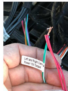
5. Install the cameras and run the video and power cables towards the radio. Make the video and power connections. The RFM-FD4 provides +12V power to the cameras.
