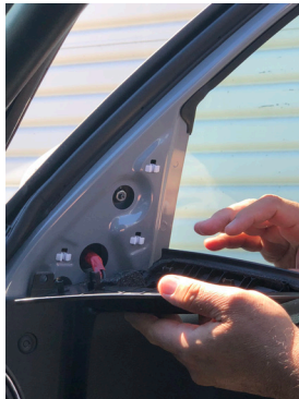
3. Use a plastic pry bar to remove the window sail. Remove the trim panel clips
