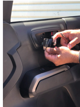
2. Remove the door unlock handle cover and remove the screw.
