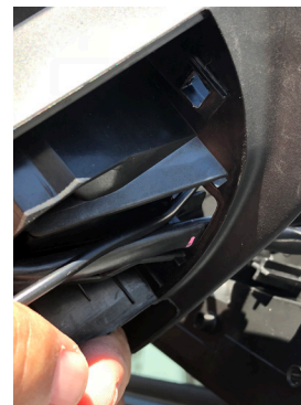
6. Tuck in the camera cable inside the cavity and snap in the CSV-TYT side mirror cover with camera.
