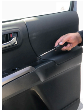
1. Remove the felt liner inside the door pull and remove the screw.
