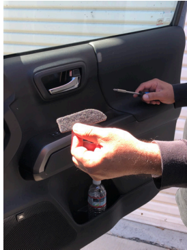
1. Remove the felt liner inside the door pull and remove the screw.
