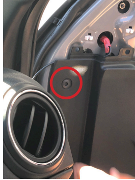
3. Use a plastic pry bar to remove the window sail. Remove the trim panel clips
