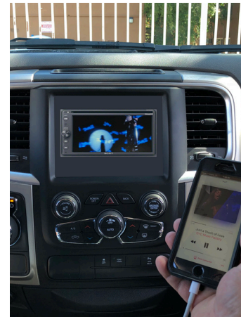
Trailer Camera Input with aftermarket radio Aux input used as an A/V Input
