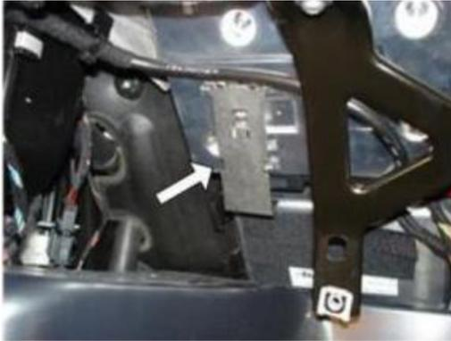
7. Remove the metal plate to unplug the LCD connector.
