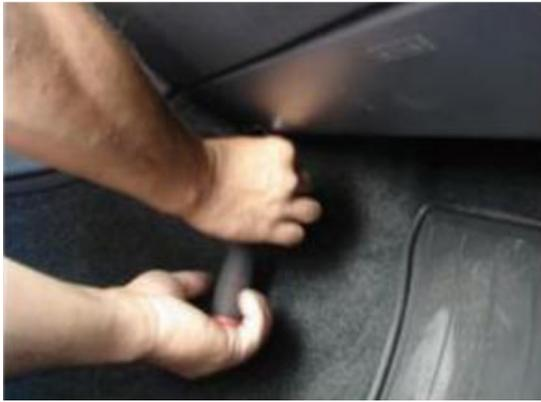
1. Remove the screws below the glove box.
