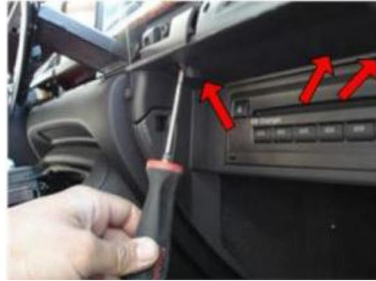
2. Open the glove box and remove the screws that hold the CD changer fascia plate.
