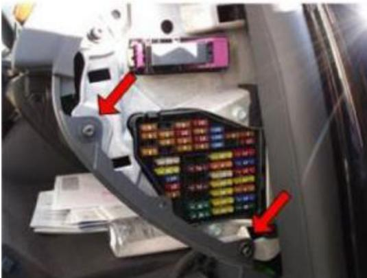
3. Remove the fuse box cover (at the right side of the dashboard) and remove the two screws.
