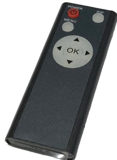
**Special Note:** To enter OSD menu please make sure Dip Switch 2 is in the ON position so that AV1 will be available. Next, enter AV1 input setting by using the push button to change inputs. Use the remote to select desired settings. Once desired settings is chosen, remove power to the module and change Dip switch 2 to the off position. Make sure the module is connected to power again and start the vehicle.
