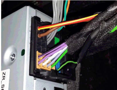
1. Unplug the Quadlock connector from the headunit.
