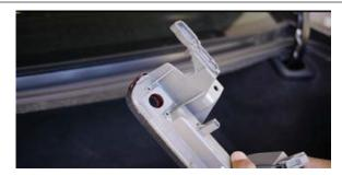
4. Insert the camera cable and the camera thru the hole but DO NOT FULLY INSERT. This will allow you to rotate the camera to the right position. Turn the ignition key to ON but do not start the engine. Put the gear in reverse and check the camera view. Adjust as necessary.
