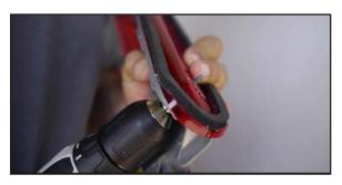
2. Continue drilling until the pilot drill bit is visible on the front side of the third brake light.
