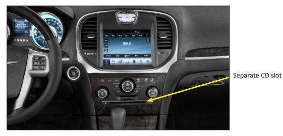
For radios without a separate CD slot (one piece radio) use part# RVCCH-75C.
