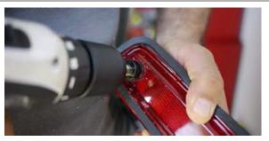
3. Turn over the third brake light assembly start drilling from the front side. Carefully drill thru the red plastic lens.
