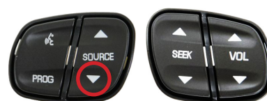
Long press of SOURCE DOWN for forced camera option 8 Button SWC
