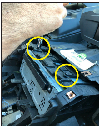
7. Remove the 2 screws holding the headunit.
