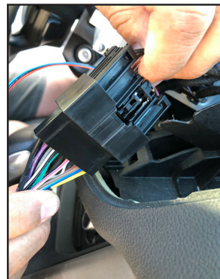
9. Mate the headunit connectors to the SWRFD-60E T-harness connectors.
