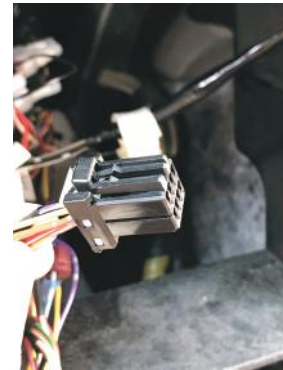
9. Note that the SWC connection is made on the 8-pin connector.
