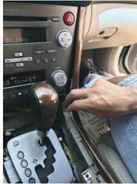
5. Remove the left and right side trims.
