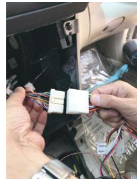
9. Note that the SWC connection is made on the 8-pin connector.
