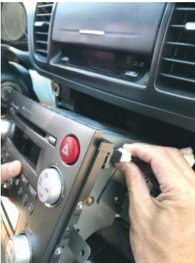
7. Unplug the hazard light connector.
