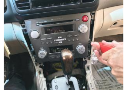
6. Remove the screws holding the radio.
