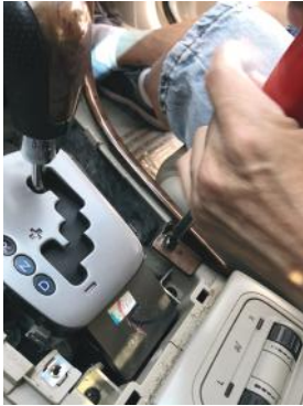
4. Remove the screws holding the left and right side trims.
