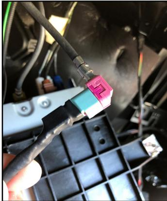
10. Plug the Pink or Gray LVDS cable to the LVDS 1 cable. Plug the other end of the LVDS 1 cable to the module LVDS OUT.
