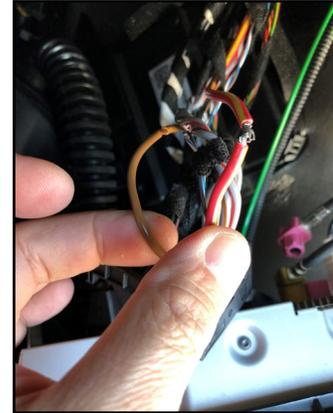
12. Tap the Red and Black wires of the VRFAD-81C harness to power & ground:
