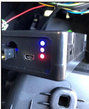
17. Test the communication. Turn on the ignition and check if LEDs are on.
