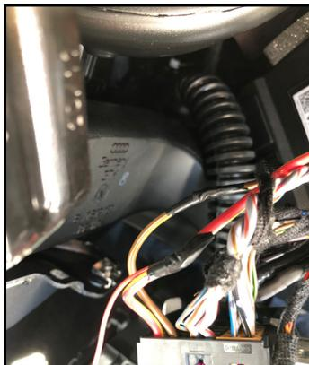
14. Install the cameras that will be used in the install. Run the camera cables towards the radio. The RCAs and camera power wires will be connected to the VRFAD-81C harness.
