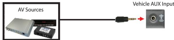
Use the GREEN wire (12V OUTPUT 2) of the VRFAD-81C harness to power the external video source (max. 1A) of the AV source.
