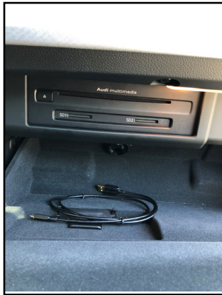
1. Installation is done behind the media player in the glove compartment.
