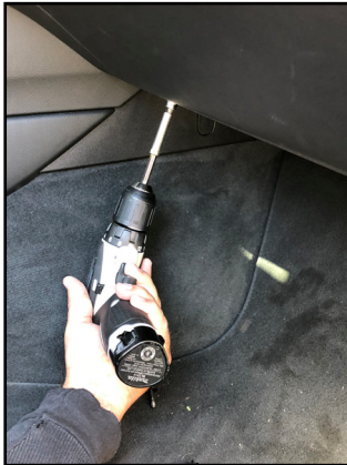
4. Remove the other screws holding the glove compartment.
