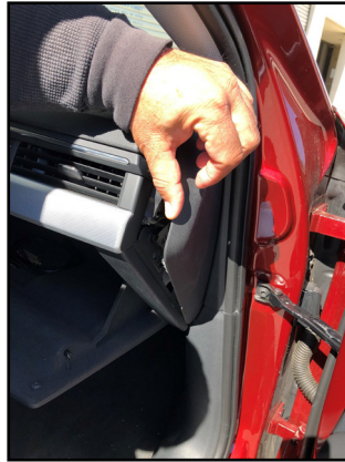
2. Remove the dashboard side panel.
