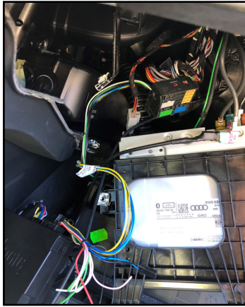
16. Plug in connectors to the VRFVW-73C module.
