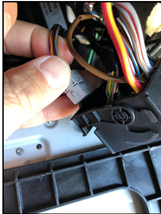
7. Unplug the Gray connector from the Quadlock connector.
