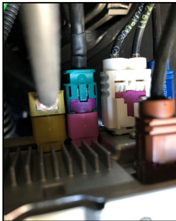
11. Plug one end of the LVDS 2 cable to the Pink LVDS port on the media player. Plug the other end of the LVDS 2 cable to the module LVDS IN.
