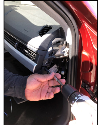
3. Remove the screw that holds the glove compartment.
