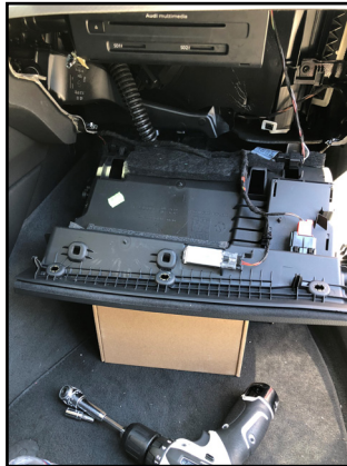
5. Pull down the glove compartment to show the media player.
