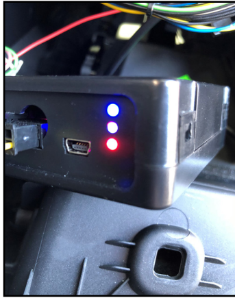
17. Test the communication. Turn on the ignition and check if LEDs are on.
