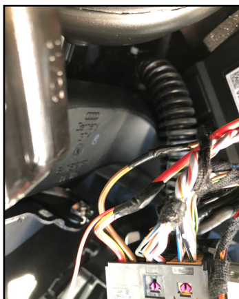
13. Tape the connections well to avoid short circuits.
