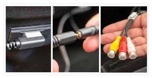
Step 5 - Connect the 8-Pin connector on the provided T-Harness to the main interface module. Make sure all your connections are firmly inserted.
