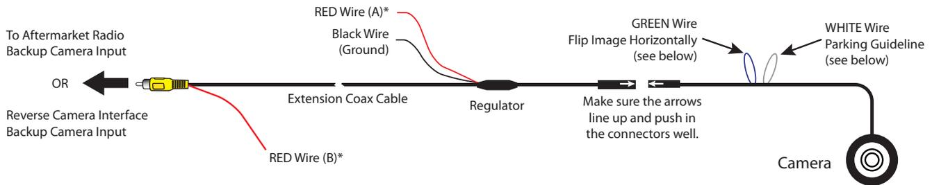
**\*NOTE:** The camera needs a +12V trigger. Power the camera at the headunit using RED Wire B or from the reverse light wire using RED Wire A. **DO NOT** connect both wires to +12V at the same time. Insulate the red wire that is not being used. Tap the Black wire to an existing ground lead, or ground Black wire securely to vehicle body metal.
