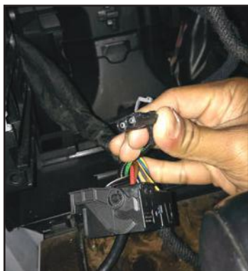
10. Unplug the 2-pin fiber optic cable from the factory Quadlock connector.
