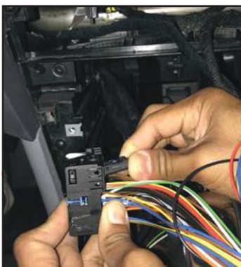
11. Plug in the 2-pin fiber optic connector to the ACPBM-77Y harness (Female side).
