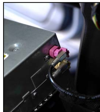
15. Unplug the PINK LVDS factory cable from the Headunit.
