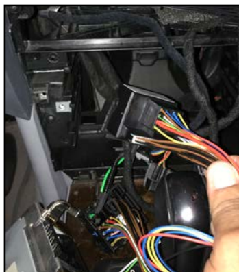
13. Plug in the female side of the ACPBM-77Y harness to the Headunit.
