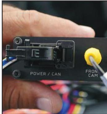
29. Connect the Power/CAN harness to the POWER/CAN input on the ACPBM-77Z module.
