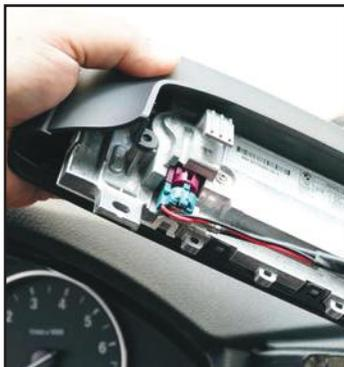
16. Connect the otherside of the CRUX LVDS Cable to the LVDS port on the LCD screen and place it to rest.
