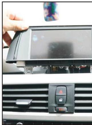
8. Remove the LCD monitor.
