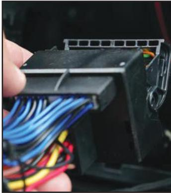
18. Connect the male side of the ACPBM-77Z vehicle harness to the factory female Quadlock connector that was originally connected to the radio.
