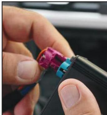
17. Funnel the Pink LVDS cable to the radio cavity and connect it to the LVDS IN port on the ACPBM-77Z module.
