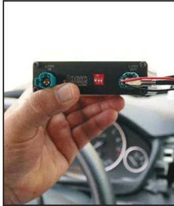
14. Insert the CRUX LVDS Cable into the LVDS OUT port on the ACPBM-77Z module.
