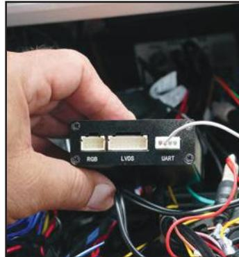
30. Connect the 4-pin connector from the Power/CAN harness to the UART port on the Smart-Play module.
