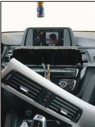
4. We must now remove the four screws behind the front panel.
