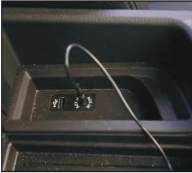
26. Connect the 3.5mm jack from the converter to the vehicle auxiliary input (AUX IN).
