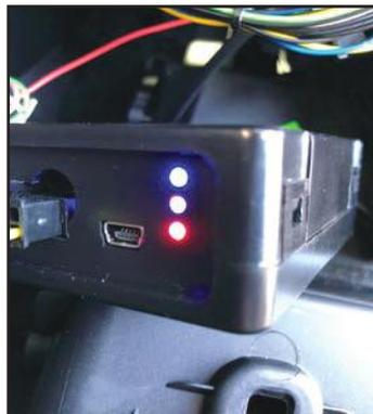
33. Test the communication. Turn on the ignition and check if LEDs are on.
