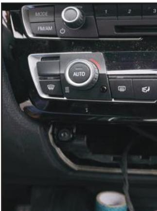
7. Remove the two torques behind the panel.
