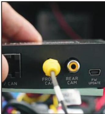
20. Plug the Video Out from the Smart-Play Power/Video harness into the FRONT CAM input on the module.
