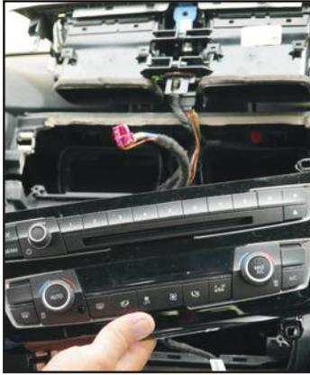
10. Remove the A/C control panel.
