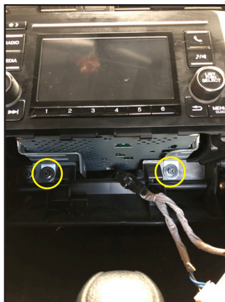
4. Remove the 2 screws holding the radio.
