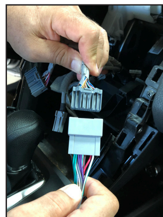
8. Plug in the SWRHN-62C T-harness and the antenna adapter to the vehicle harness.
