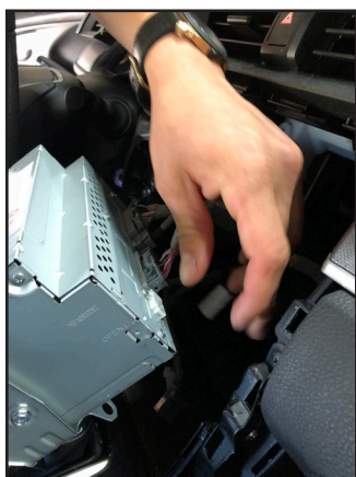
6. Unplug the radio connectors.
