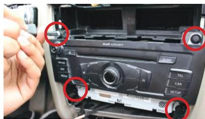
7. Remove the 4 screws holding the radio.
