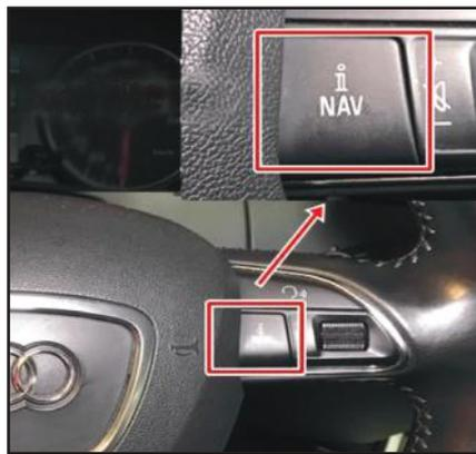
To enter and exit the Smart-Play mode, press the NAV button on the steering wheel controls for 2 seconds.
