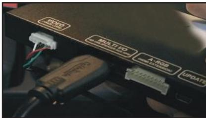
25. Plug in the 4K HDMI cable to the ACPAD-01W module.
