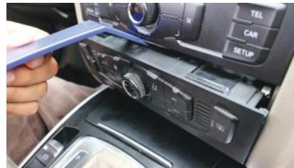
5. Remove the AC control module with a plastic pry tool.
