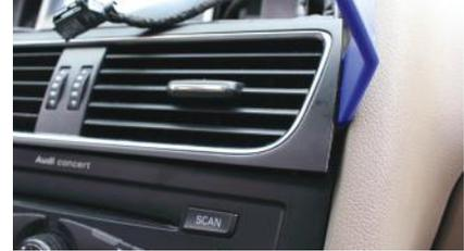
3. Carefully remove the air vent using a plastic pry tool. Work your way around the vent to avoid damaging it.
