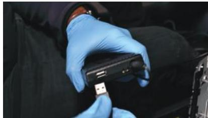
26. Plug in the USB extension cable to the Smart-Play module if wired CarPlay /Android Auto is desired.
