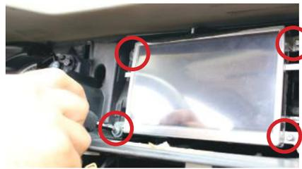
9. Remove the OEM screen by removing the 4 T-20 torx screws on each corner.
