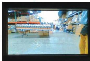
The front Camera will automatically show on the screen when the gear is put to Drive from Reverse. Set the delay time on the OSD menu. Delay time can be set from 1 to 60 seconds after a putting the car to drive from reverse.
