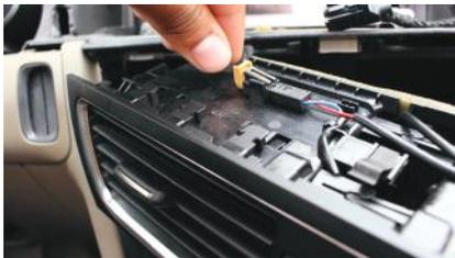
4. Unplug the 2-pin connector behind the air vent.
