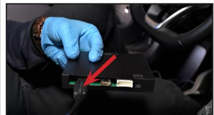
18. Plug the other end of the 4K HDMI cable to the ACPMB-45 module HDMI port.
