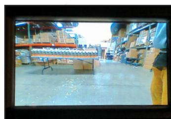
The front Camera will automatically show on the screen when the gear is put to Drive from Reverse. Set the delay time on the OSD menu. Delay time can be set from 1 to 60 seconds after a putting the car to drive from reverse.
