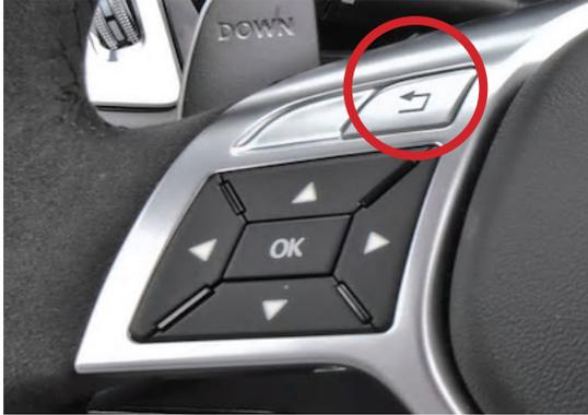
To enter and exit the Smart-Play mode, press the back button
