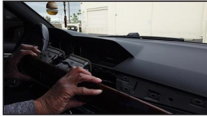
2. Carefully pull out the dash trim. It is held in place by multiple clips.
