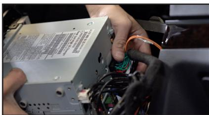
10. Plug the ACPMB-45 Quadlock connector to the radio.
