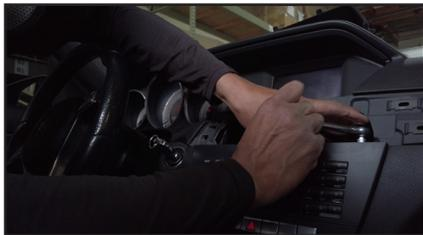
4. Remove the 2 Torx screws holding the radio.
