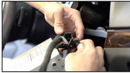
8. Plug the fiber optic cable to the same location on the ACPMB-45 Quadlock T-harness.
