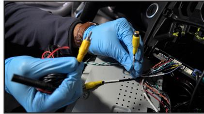
14. Install the front and rear cameras (if applicable) and power using the power wires provided.
