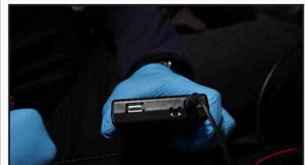
21. Plug one end of the Aux cable to the Smart-Play module and other end to the factory AUX port.
