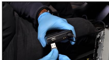
19. Plug in the USB extension cable to the Smart-Play module.
