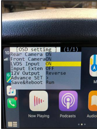
After plugging in the OSD controller, navigate down to **LVDS Input** and set to ON. Push RIGHT button to go to the next menu.
