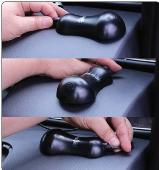
20. With the ignition turned to ACC, put the vehicle in reverse. Turn on the monitor and find the best direction for the receiver turning it until you see atleast 3 bars on the monitor.
