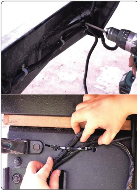
17. Organize the cables using zip ties and cable clamps.
