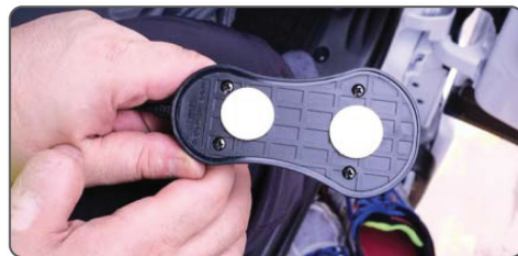
19. Attach the double sided adhesive tape under the receiver. Do not remove the bottom liner of the double sided tape yet.
