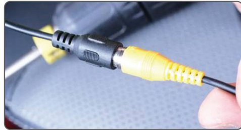
18. Connect receiver's red wire to ACC and black wire to ground. Plug the Yellow video RCA to the monitor (not included).
