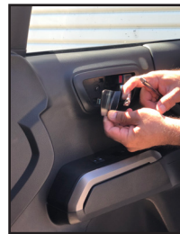
2. Remove the door unlock handle cover and remove the screw.
