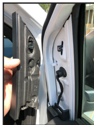
5. Use a hooked pick tool to remove the OEM side mirror cover. Fish the camera cable through the hole.
