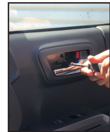
2. Remove the door unlock handle cover and remove the screw.
