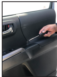
1. Remove the door pull and remove door panel the screws.
