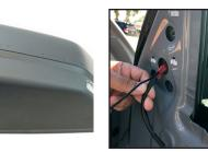
5. Use a hooked pick tool to remove the OEM side mirror cover. Fish the camera cable through the hole.
