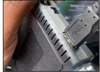
22. Plug in the USB extension cable and run it to an easily accessible location.
