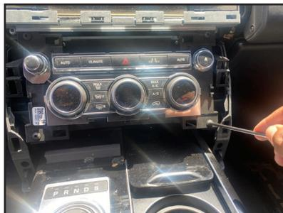
5. Remove the 4 Torx screws holding the AC control panel and unplug the connector.
