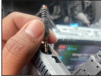
21. Mount the microphone to the desired location and run the cable towards the Smart-Play module. Plug it to the microphone input.
