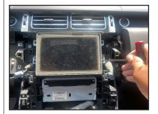
8. Remove the 4 Torx screws holding the touch screen.
