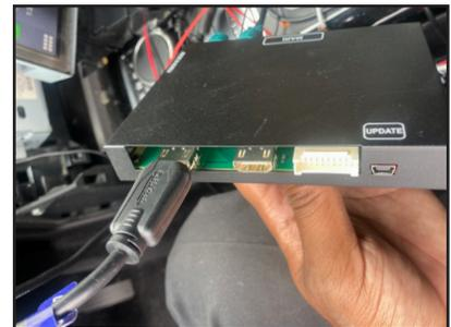
15. Plug in one end of the HDMI cable to the left HDMI port on the module.
