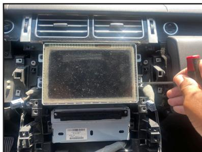
8. Remove the 4 Torx screws holding the touch screen.
