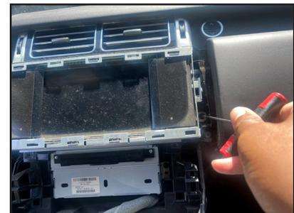
6. Remove the Torx screws holding the left and right radio control panels.
