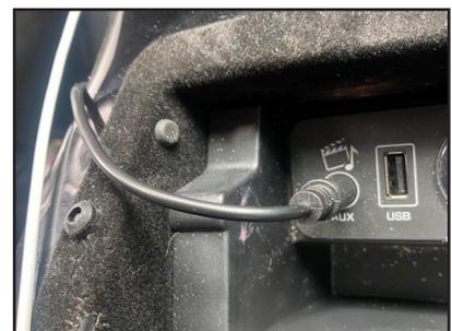
18. Plug the other end of the 3.5mm Aux cable to the factory Aux input.
