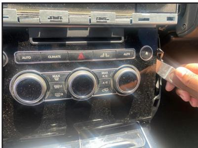
4. Carefully remove the AC control panel using a pry tool.
