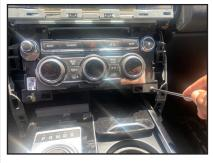
5. Remove the 4 Torx screws holding the AC control panel and unplug the connector.
