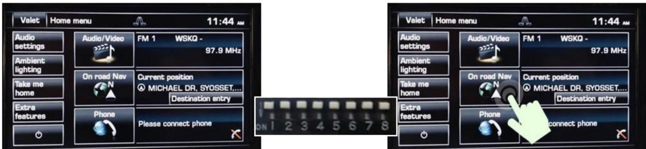
For vehicles with factory navigation set DIP#5 to OFF (up) before powering the module.
