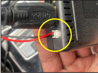
20. Plug in the Smart-Play power plug and tap to 12V ACC and Ground.
