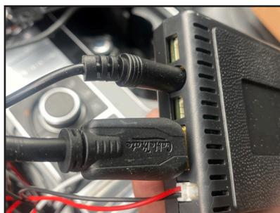
17. Plug in the 3.5mm to 3.5mm Aux cable to the Smart-Play module.
