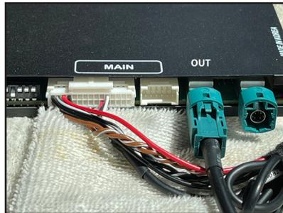
14. Plug the LVDS connector of the GVIF video cable to "OUT" port on the module.
