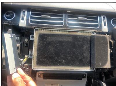
7. Remove the radio control panels and unplug the connectors.
