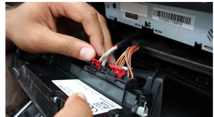
6. Unplug the 2 connectors behind the AC control module.
