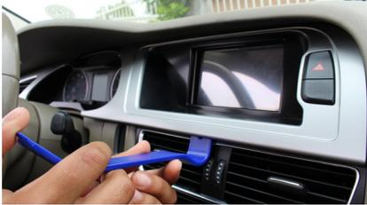
1. Carefully remove the dash panel trim with a plastic pry tool. Work your way around the panel to avoid damaging it.
