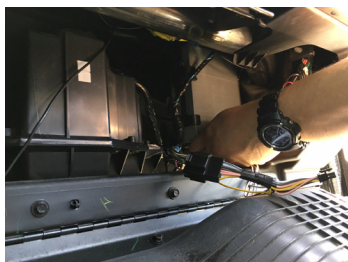
4. Plug the other 16-pin connector of the BTS-GM1X harness to the XM tuner.
