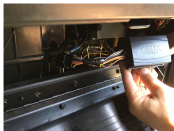
5. Plug the 12-pin Molex connector to the BTS-GM1X module.
