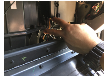
6. Use cable ties to secure the module.
