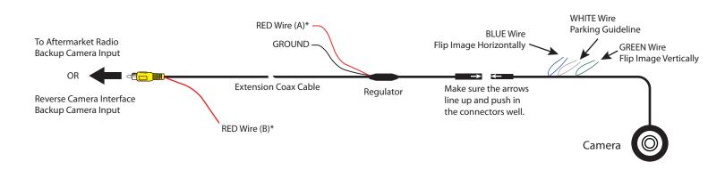
\*NOTE: To power the camera, use RED Wire A or B. If tapping power from the radio or RVC Interface, make sure to insulate RED Wire A to avoid it from shorting. If you will be tapping power from the reverse light +12V, insulate RED Wire B to avoid it from shorting. With either connection the Black GROUND wire needs to be connected to a solid chassis ground. For vehicles with manual transmission, we recommend tapping +12V power from the reverse light.
