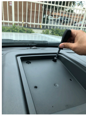
1. Lift the rubber mat on the dashboard upper tray and remove the 2 screws.
