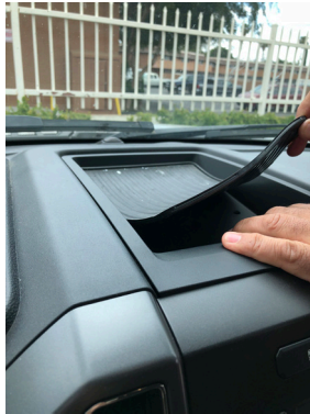
1. Lift the rubber mat on the dashboard upper tray and remove the 2 screws.
