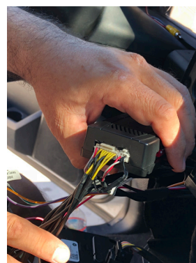
6. Plug the white, 18-pin connector of the T-harness to the RFM-FD8 module.
