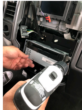
4. Remove the factory screen, unplug the male connector and plug it into the RFM-FD8 T-harness. Plug the other end of the T-harness to the screen.
