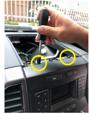
2. Remove the tray and remove the 2 screws holding the radio bezel.
