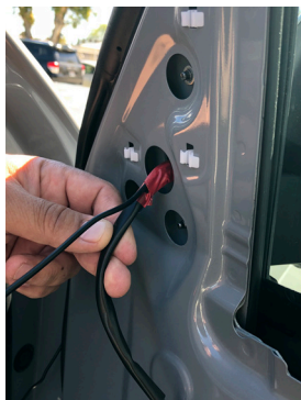
5. Use a fine hooked pick tool to remove the OEM side mirror cover. Fish the camera cable through the hole.
