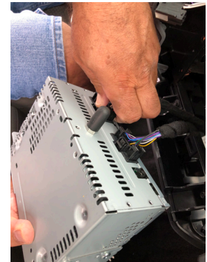
4. Remove the factory screen, unplug the male connector and plug it into the RFM-FD8 T-harness. Plug the other end of the T-harness to the screen.
