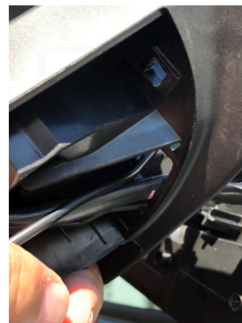
6. Tuck in the camera cable inside the cavity and snap in the CSV-FD15 side mirror cover with camera.
