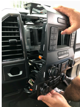
3. Carefully pull out the radio bezel. This is held by multiple clips.
