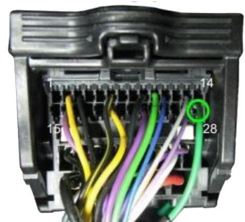
GREEN wire Single CAN wire PIN# 28
