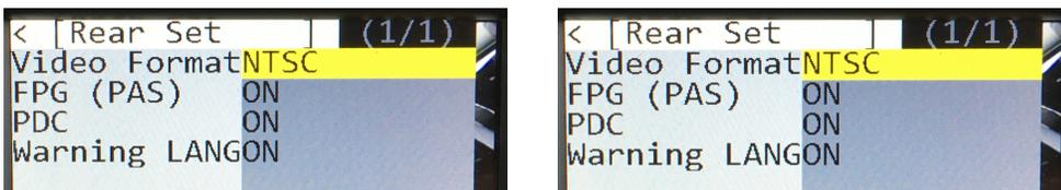
To turn ON the Dynamic Parking Guide Lines, go the Rear Input > Rear Set and turn ON Warning LANG. Go back to the root menu and Run Save&Reboot. Remember to unplug the OSD Control Pad otherwise the unit will not function properly. Set the parking brake on, start the car, put the gear in reverse, turn the steering wheel all the way to the left and all the way to right then put it in the center. The ACPLX-12Z will calibrate automatically.
