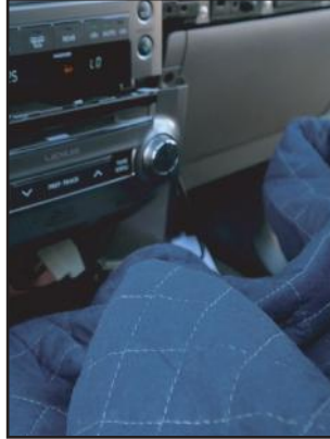
14. Place a protective cloth on top of the shifter to prevent damage.
