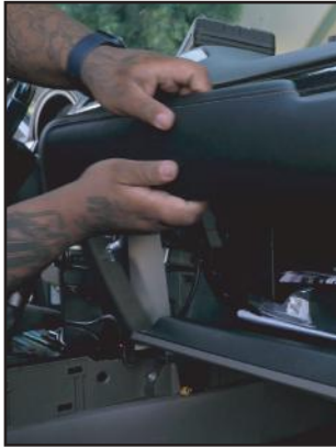
4. Pull out the center console from the back cup holder.
