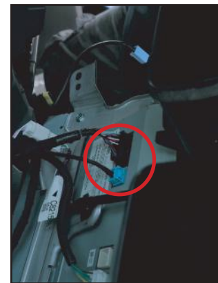
21. Remove the black and blue connectors from behind the panel.
