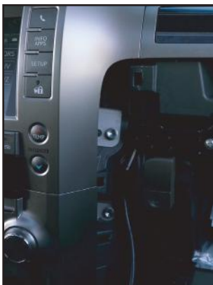
10. Remove the two 10mm bolts on the right.
