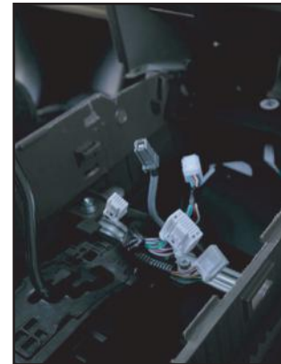
9. Now you can remove the center console by disconnecting its connectors.
