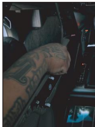
2. Remove the right & left leather side trims along the center console.
