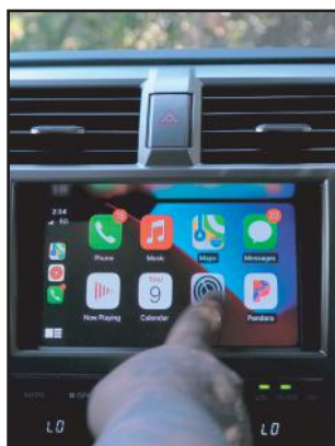
26. Connect your phone via lightning cable and test the features for wired CarPlay/AA or wireless Carplay/AA.
