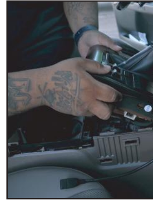
6. Plug the 62 pin t-harness provided to the factory radio.
