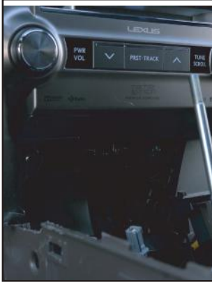
13. Remove the two remaining 10mm bolts.
