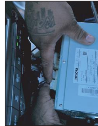
18. Then insert the other ends of the CRUX harness in to the radio.
