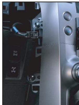
11. Remove the two 10mm bolts on the left.
