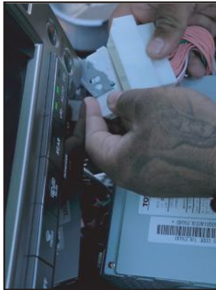
17. Connect these two connectors to the CRUX harness provided in the kit.
