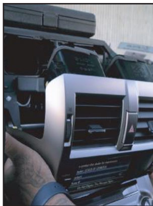
20. Remove the factory display panel.
