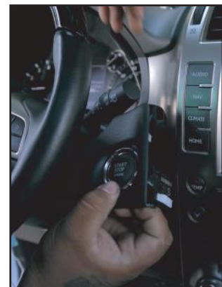
3. Remove and unplug the start button panel.
