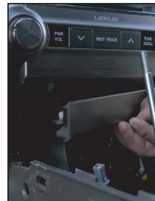
12. Remove the plastic trim hiding the two remaining 10mm bolts.
