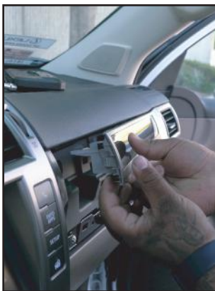
19. Pry open only the left side of the following trim to make room.
