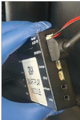
11. Plug in the power plug, 4K HDMI cable and the 3.5mm Aux cable to the Smart-Play module. Run the 3.5mm Aux cable to the factory Aux input location
