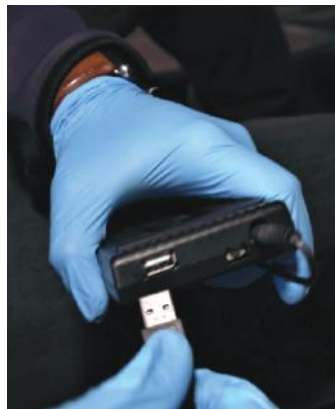
12. Plug in the USB extension cable and mic to the Smart-Play module. Run the USB extension cable to an accessible location. Run the mic cable to the A pillar.
