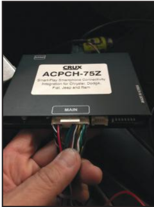
8. Plug in the main harness to the ACPCH-01W module.
