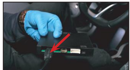
18. Plug the other end of the 4K HDMI cable to the ACPMB-45W module HDMI port.
