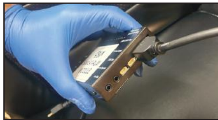
16. Plug in the 4K HDMI cable provided with the kit to the Smart-Play module.
