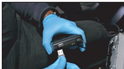
19. Plug in the optional USB extension cable to the Smart-Play module for wired AA/ Carplay
