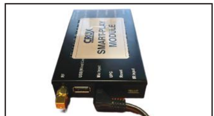
21. Plug the AMI-3.5 MM Aux adapter cable to the factory AMI port and the other end to the Smart-Play module Line Out.
