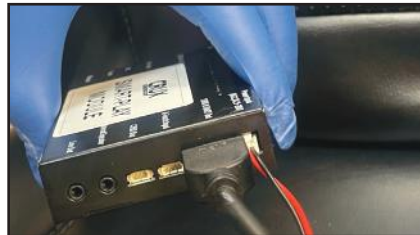
17. Plug the 2 pin power wire connector to the Smart-Play module.
