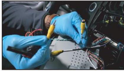
14. Install the front and rear cameras (if applicable) and power using the power wires provided.
