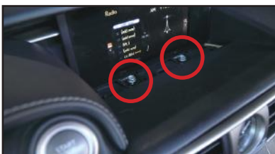
10. Use a pry tool to remove the trim in front of the screen. Remove the screws.
