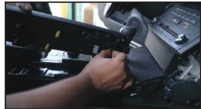
3. Remove the Jog Wheel console and unplug the harness.
