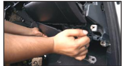
6. Remove the gear shifter panel and set aside.
