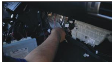
8. Remove the headunit and the climate control panel.
