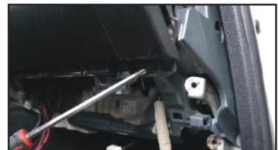
9. Remove the glove box to gain access for mounting the ACPLX-12YW modules.
