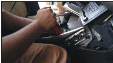
2. Remove the right and left side trim along the center console.
