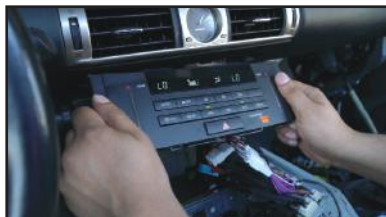
8. Remove the headunit and the climate control panel.
