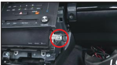
7. Remove the screws holding the headunit.
