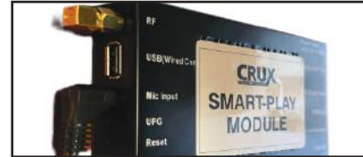
15. Plug in the power plug, HDMI, mic, aux-in, and USB extension to the Smart-Play module.
