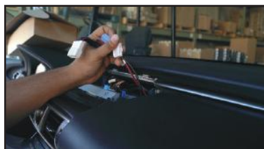
11. Run the ACPLX-12YW harness from the glove box area to the screen.
