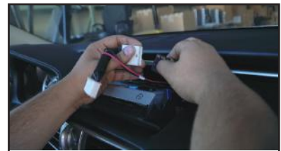
9. Remove the glove box to gain access for mounting the ACPLX-12YW modules.
