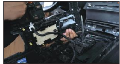
6. Remove the gear shifter panel and set aside.
