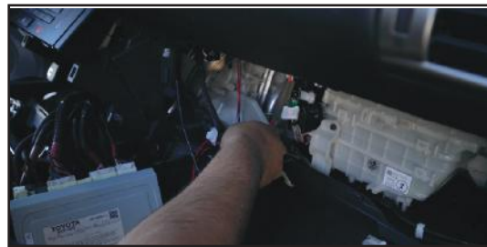
16. Mount the ACPLX-12YW modules behind the dash and test before reinstalling the whole dash area.
