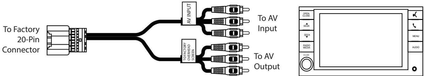
1. Remove the OEM radio and plug the CRUX 2444A's 20 pin connector to the vehicle's 20 pin factory RSE connector at the factory radio location. Use one of the Crux parts listed in the Note section.
