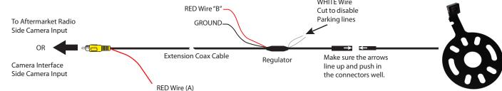
\*NOTE: Tap RED Wire A or RED wire B to the radio or camera interface +12V camera power output and the black wire to chassis ground. DO NOT CONNECT BOTH RED WIRES AT THE SAME TIME! Only one red wire gets connected depending on installation.
