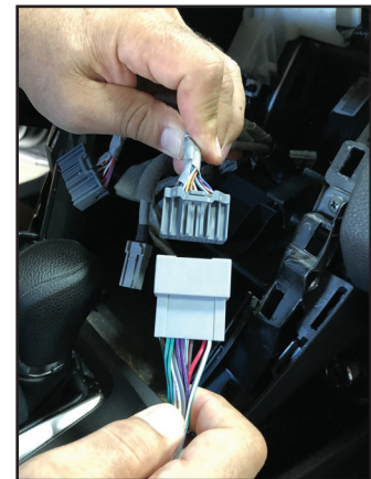
8. Plug in the SWRHN-62C T-harness and the antenna adapter to the vehicle harness.
