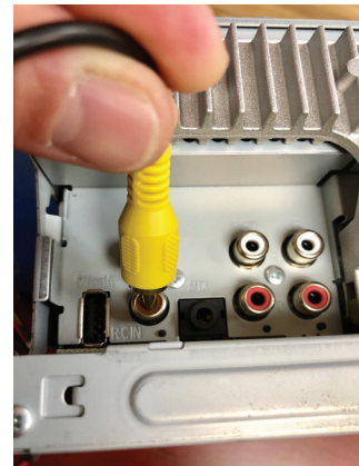
7. Make the connections between the SWRHN-62C harness and the aftermarket radio harness. Plug in the backup camera RCA
