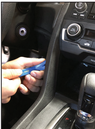
1. Using a plastic pry tool, remove the left and right dash trims.
