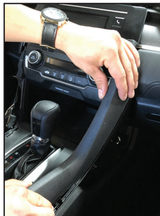
1. Using a plastic pry tool, remove the left and right dash trims.
