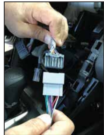
8. Plug in the SWRHN-62S T-harness and the antenna adapter to the vehicle harness.
