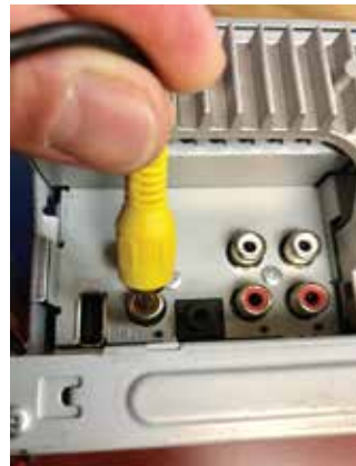
7. Make the connections between the SWRHN-62S harness and the aftermarket radio harness. Plug in the backup camera RCA
