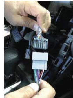
8. Plug-in the SWRHN-62S T-harness and the antenna adapter to the vehicle harness.
