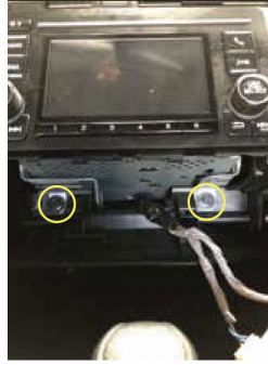
4. Remove the 2 screws holding the radio.
