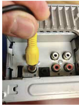
7. Make the connections between the SWRHN-62S harness and the aftermarket radio harness. Plug-in the backup camera RCA.
